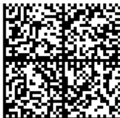
Figure 9: Digital Seal for address sticker containing the passport number, official municipality code number and residential address signed with brainpoolP224r1 curve
