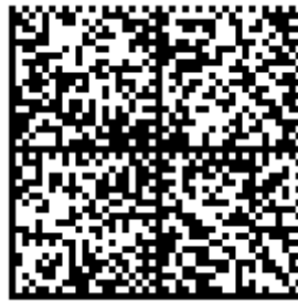
Figure 6: Digital Seal of a SIC containing: social insurance number, first name, last name, name at birth, issuing date and an elliptic curve signature
