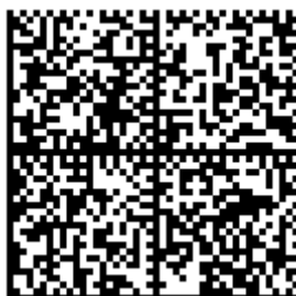
Figure 8: Digital Seal for VISA sticker containing MRZ, Duration of Stay and passport number signed with brainpoolP224r1 curve
