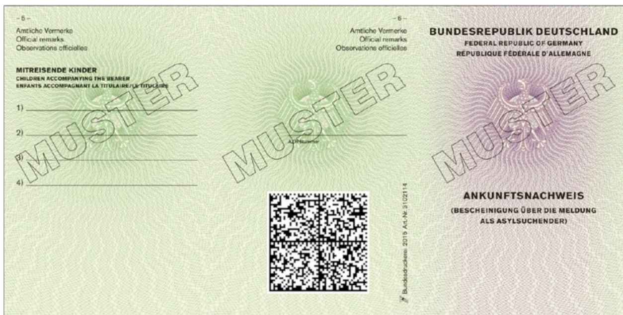
Figure 5: Front side of the Arrival Attestation Document encoded in an DataMatrix bar code containing the MRZ, AZR number and the elliptic curve signature
