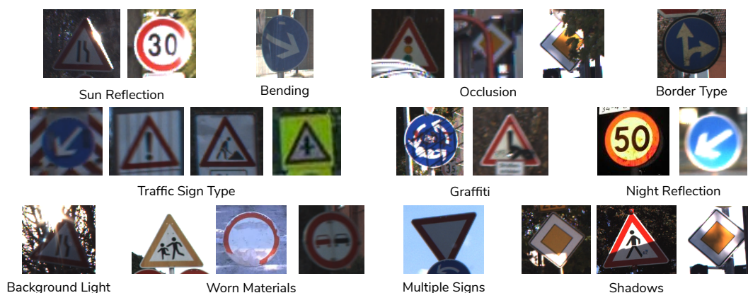
Figure 13: Real world examples of properties that are relevant for traffic sign classifiers.
