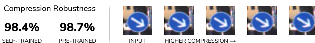
Figure 10: Robustness to using JPEG compression. For pre-trained model the images have resolution 299 \times 299 and compression quality was set between 90 to 20. For self-trained model, the images are smaller with resolution only 32 \times 32 and therefore we used higher compression quality from 90 to 80.
